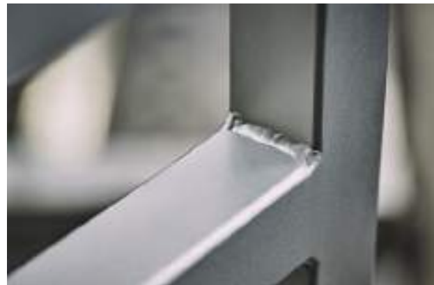
III. left assembly production of stainless steel components (TIG welding) III. top hygiene requirements – edges to prevent dirt accumulation III. middle primate-safe cage closures III. bottom clean and corrosion resistant weld seams (TIG-welding)
